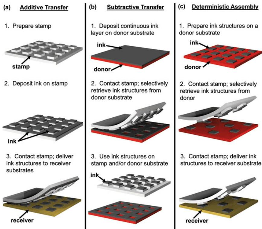
**Fig. 1** Schematic of three transfer printing schemes. **a** Additive transfer delivers ‘inked’ materials at regions that come into contact with the target substrate. **b** Subtractive transfer results in patterned material on donor substrate, as well as inked material on stamp for additive transfer, as in (a). **c** Deterministic assembly involves removal of selected structures from the donor substrate, followed by a printing onto a receiving substrate. Reprinted with permission from [16]
