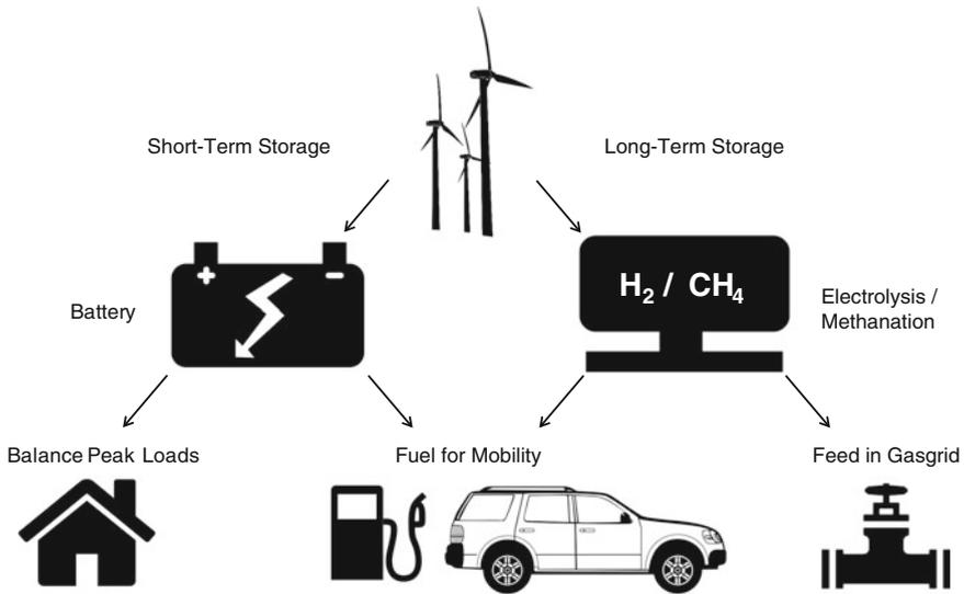
**Fig. 5** Combined system of wind energy and storage technologies
