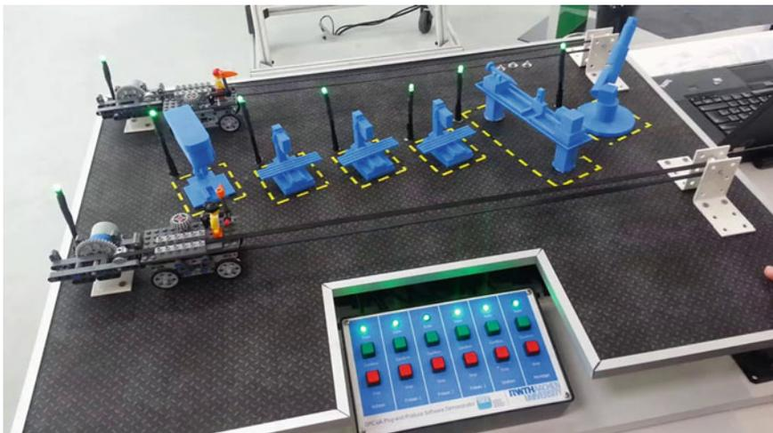
**Fig. 4** Agent-based demonstrator simulating virtual production processes for intelligent agent-based manufacturing organization
