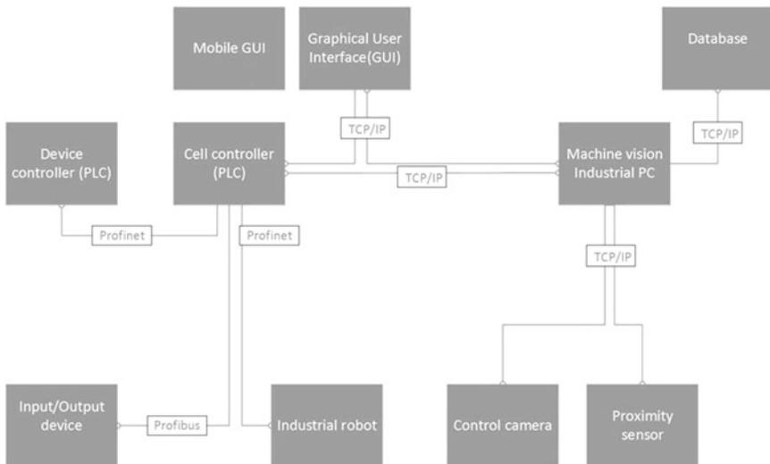
Fig. 3 Communication structure of automation
