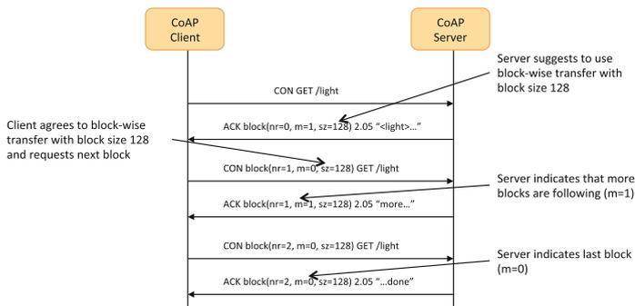
Fig. 9 A CoAP client requests the resource light and receives a block-wise answer. The client requests more blocks until the server informs the client that no more blocks are available
