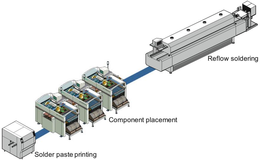
Fig. 6 In-line structure of an SMD assembly line
