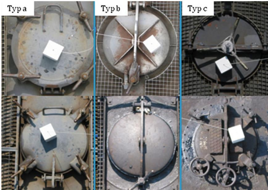
**Fig. 1** Dome cover closure types
