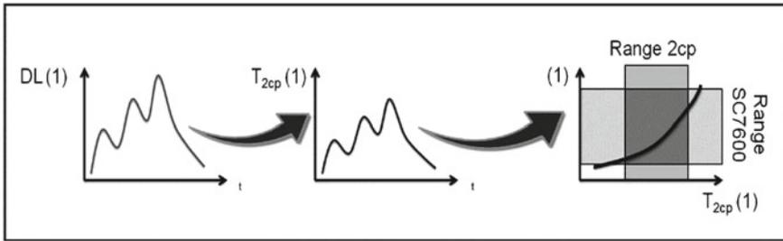
Fig. 4 Concept for the calibration of infrared camera data [7]
