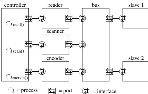
Fig. 11 A part of a JPEG encoder
