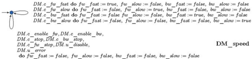
Fig. 11 Automaton for observer of drive commands
