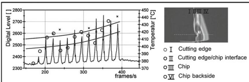
Fig. 5 Reducing calibration variance via location-referenced measurements [7]
