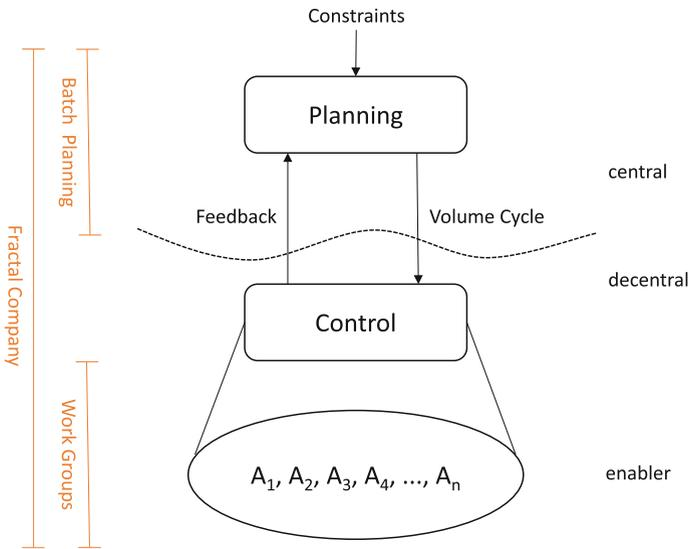
**Fig. 4** Conceptual approach of decentralized planning and control based on CPS. The main basic principles can be found on the *left side* of the figure. The concept of fractal companies represents the thematic framework. Batch planning methods help to define the number of orders handed over to working group consisting of CPS and human workers who organize their tasks
