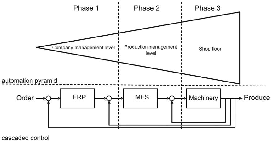
**Fig. 4** Automation pyramid in comparison with cascaded control
