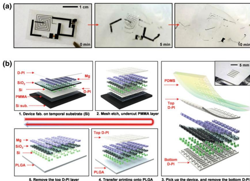
**Fig. 6** **a** Optical images show the dissolution sequence of a proof-of-concept device in deionized water. Reprinted with permission from [81]. **b** Materials and procedures to fabricate dissolvable electronic devices on biodegradable substrates. Reprinted with permission from [85]
