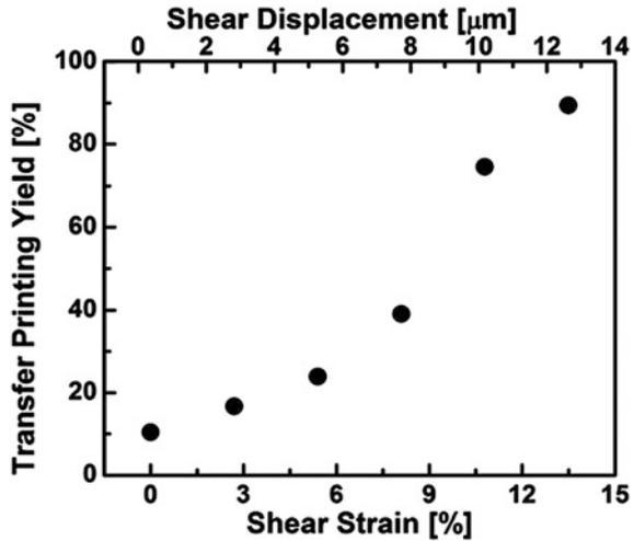
linearly with an increase in shear displacement. In addition, transfer yield significantly increases with an increase in shear displacement. With an increase in shear strain up to 14 %, a ten-fold increase is observed in yield (Fig. 4). Hence, shear-enhanced transfer printing, in comparison with conventional TP, has a higher efficiency and therefore facilitates the printing of inks onto complex receiver substrates.
