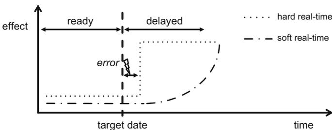
Fig. 3 Illustration of the hard and soft real-time requirement [34]
