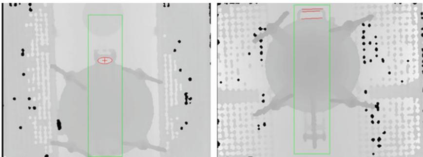
**Fig. 2** Examples for identification of the orientation of the dome cover
