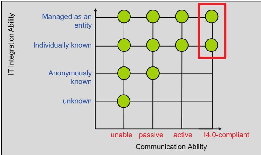
Fig. 6 Classification of an I4.0 component According to [44]
