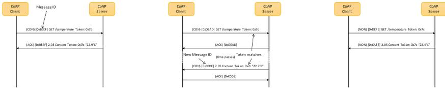
**Fig. 8** *Left* A CoAP request that is directly answered by piggybacking the response on the ACK. *Middle* A delayed response to a request, please note the use of a fresh Message-ID and the same Token. *Right* A non-confirmable request and response, using different Message-IDs but the same Token. (cf. [61])
