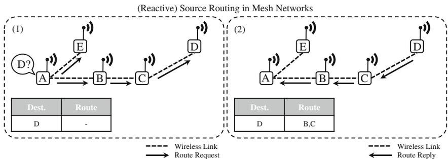
**Fig. 4** Route discovery in reactive mesh routing. Node A requests a route to D, which is discovered and after the route reply from D (temporary) stored in A's routing table
