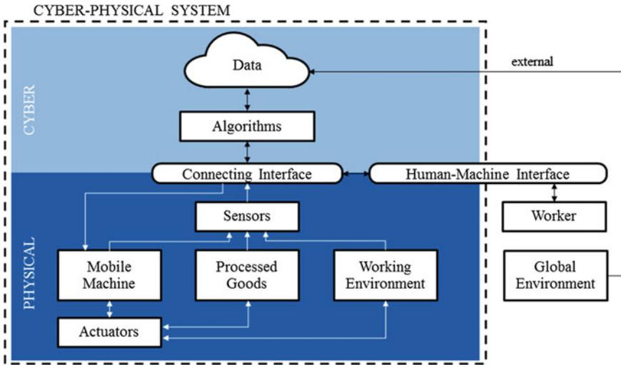
Fig. 2 System boundary of a CPS in mobile machines
