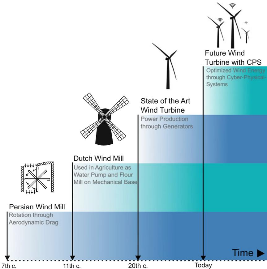
**Fig. 1** Development of wind turbines
