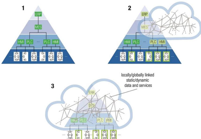
**Fig. 3** Gradually replacement of the classical automation pyramid [26]
