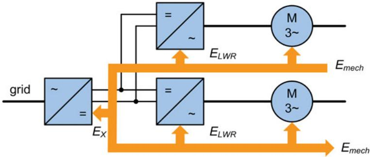
Fig. 4 Two motors connected to a DC circuit
