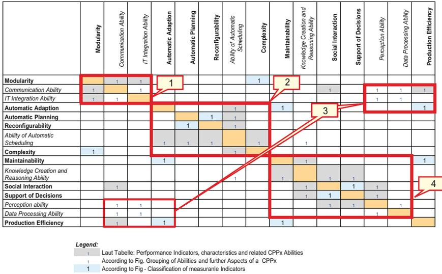
**Fig. 10** Clustered DSM matrix of measurable performance indicators and technological abilities (the following Abilities are not displayed for the reason of simplicity: generalization ability, specialization ability and usability)
