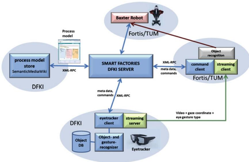
**Fig. 4** Intelligent user interface architecture
