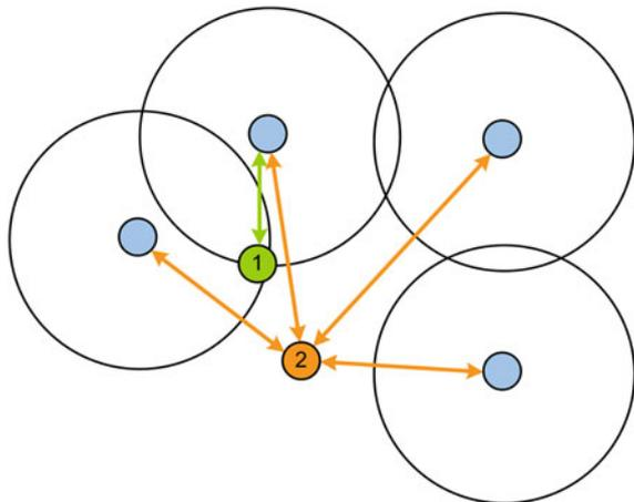
The PCA can also be used for predictive analytics. For this, two core distances have to be used. Crossing the first threshold, a warning is given, crossing the second threshold, an anomaly is signaled.
