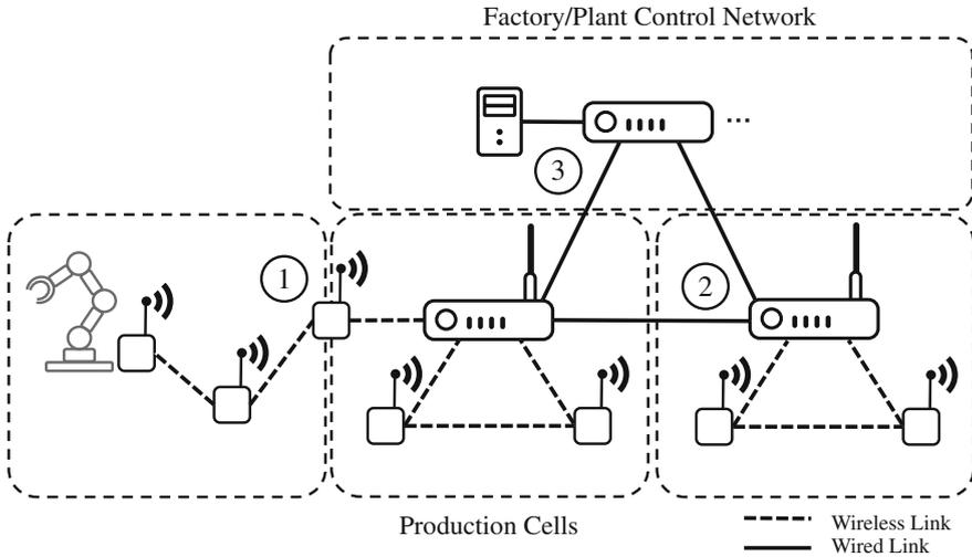
**Fig. 3** Communication scenarios between production cells within the factory or across the whole factory site. Individual cells are either (1) connected through wireless links or (2) by multi-homed gateways, connected via a wired link. Ultimately, these are connected to (3) the control and automation network of the factory
