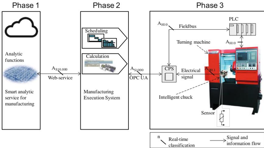
Fig. 5 CPS for a turning machine
