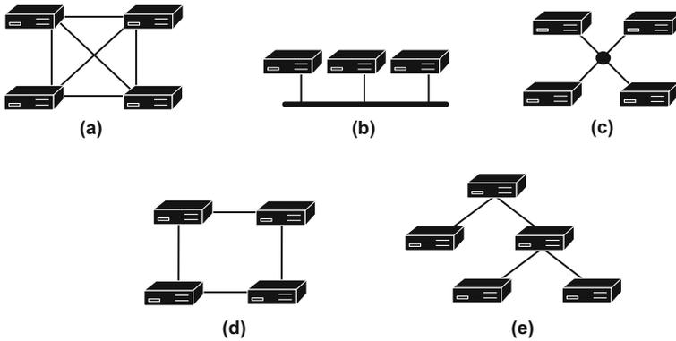
**Fig. 3** Fundamental topologies of communications network: **a** full-mesh, **b** bus, **c** star, **d** ring, and **e** tree
