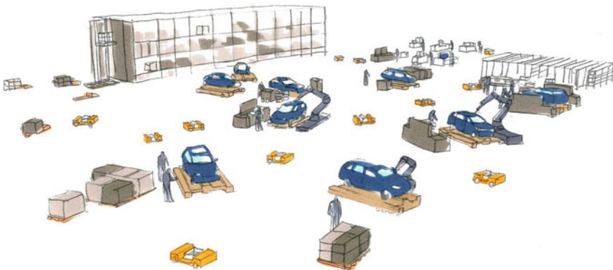
**Fig. 1** The vision of SMART FACE: decentrally and autonomously acting units (e.g., assembly stations, automated guided vehicles, industrial robots, etc.) are responsible for transporting and producing goods on a self-organizing shop floor. Human workers are still an important part since they exhibit the largest flexibility that is an important enabler for the concepts
