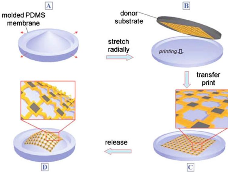
**Fig. 5** Deployment of electronic systems onto an arbitrary curvilinear surface via transfer printing. Reprinted with permission from [68]
